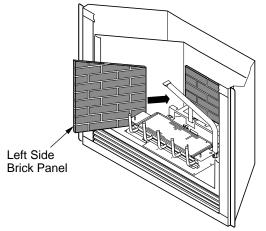
Figure 44 - Installing Left Side and Top Brick Panels
